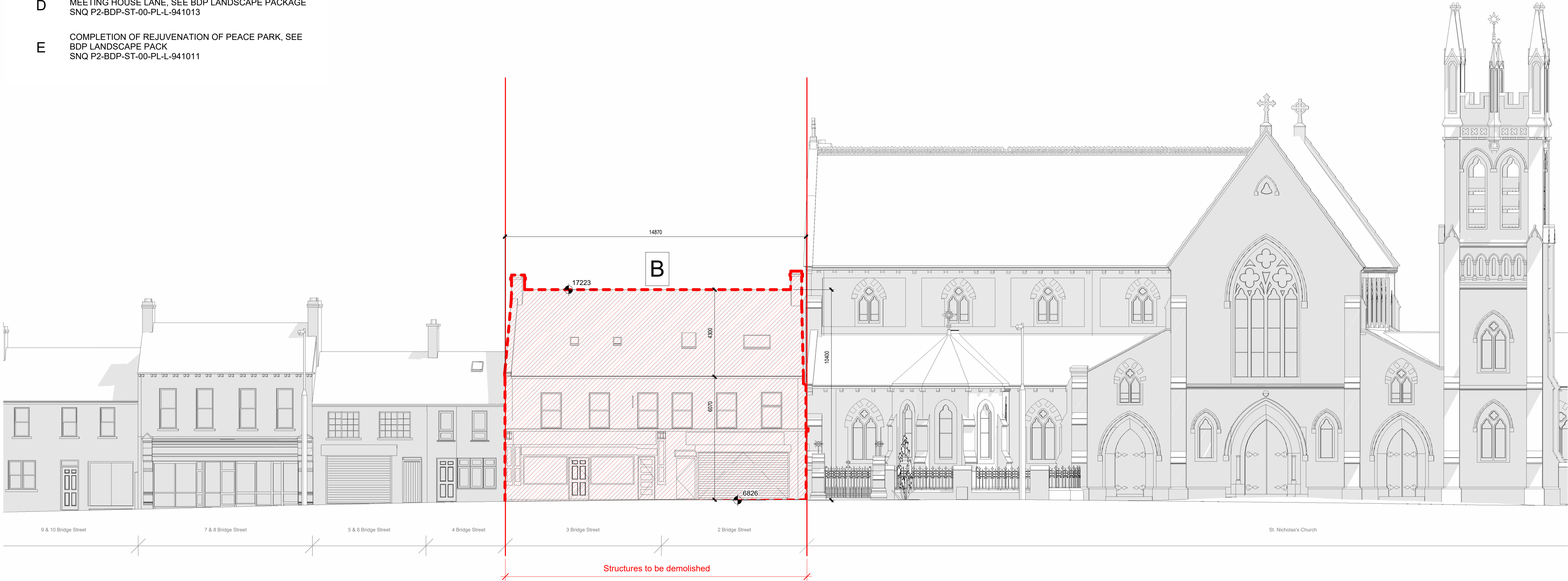
Demolition Elevation Existing Bridge Street 1:100
