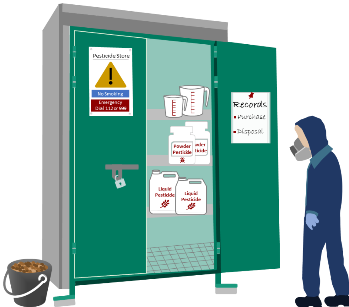
Figure 19: Pesticide storage requirements.
