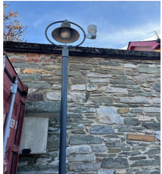
Rainwater gauge, to measure rainwater at the site for use with the proposed rainwater harvesting system.
