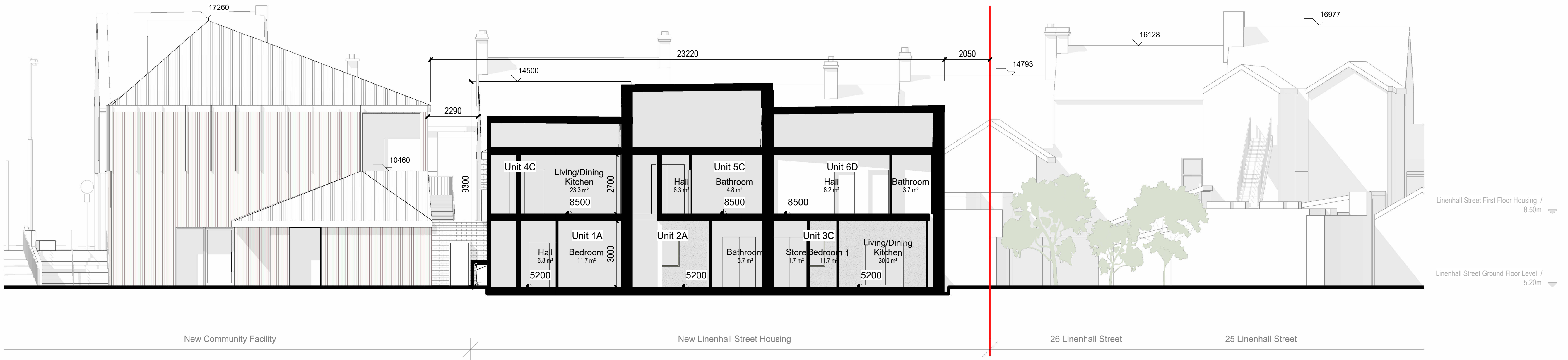
Residential Unit Proposed Section DD 1:100
