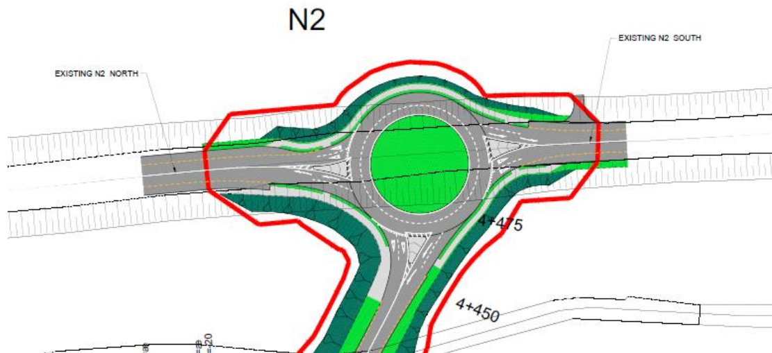
Figure 3-7 N2 Roundabout Junction
