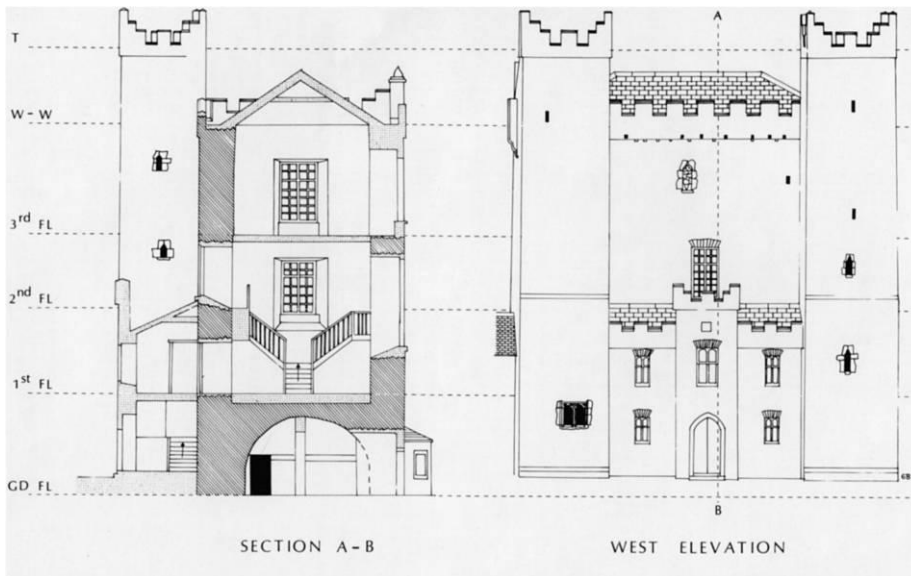
Fig. 5: Ardee Castle, section and elevation from Murtagh
