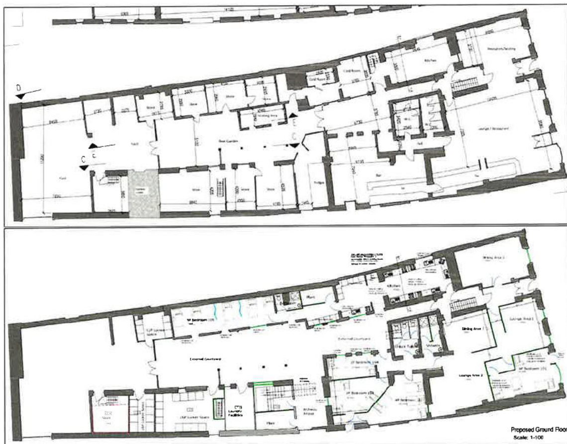
Figure 11.0 Existing (top) and proposed (bottom) ground floor plans. We note minor changes to the fenestration details and external openings at this floor level.
