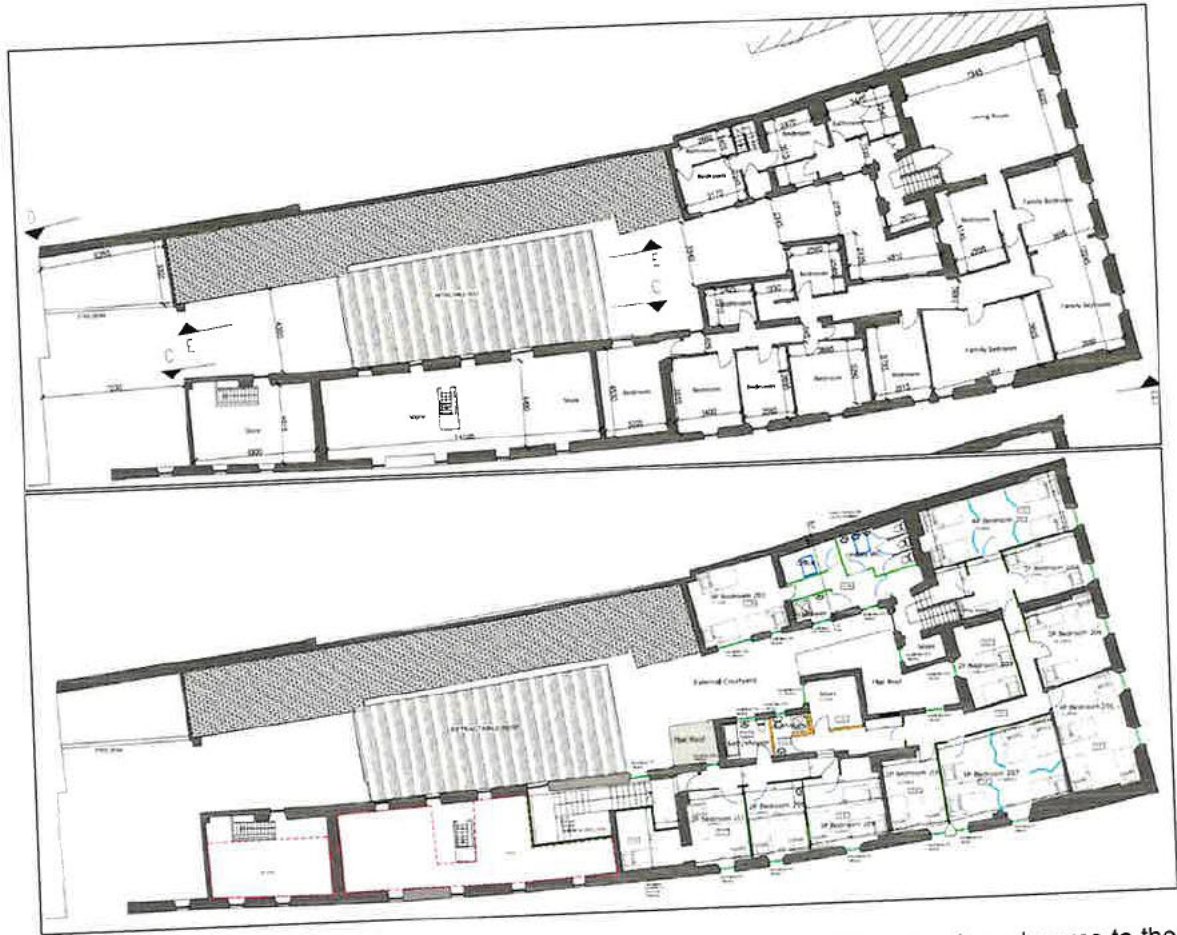
Figure 12.0 Existing (top) and proposed (bottom) first floor plans. We note minor changes to the fenestration details and external openings at this floor level.
