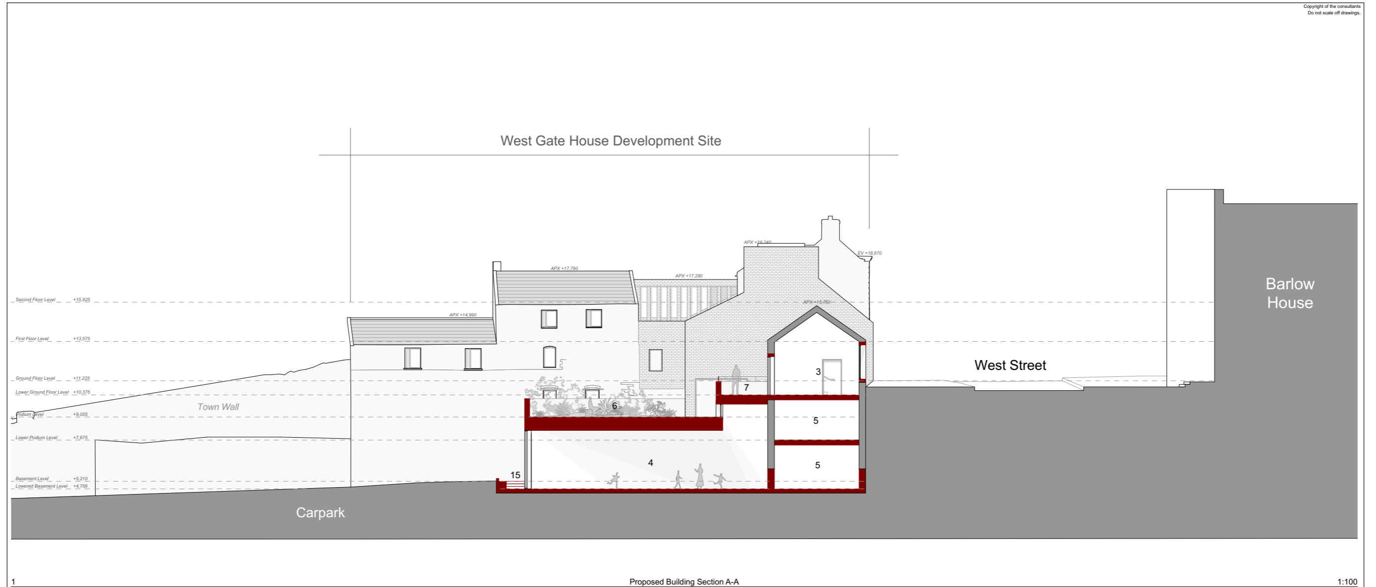
1 Proposed Building Section A-A 1:100
