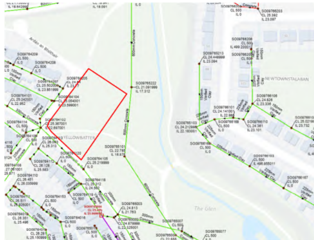
Plate 17. Extract of Municipal drainage mapping illustrating the Combined Municipal drainage network in the vicinity of the site (note red rectangle represents the approximate outline of the site)
