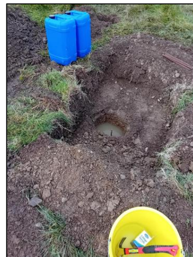
Supervised Percolation Test
