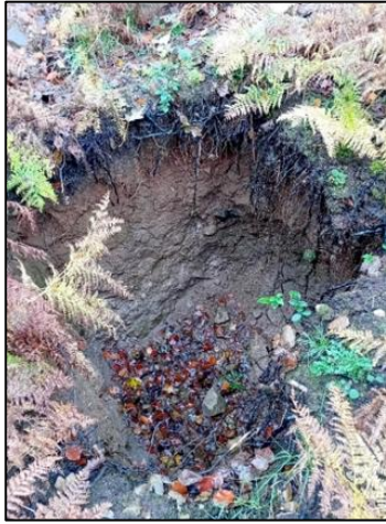
Trial Hole Inspection
