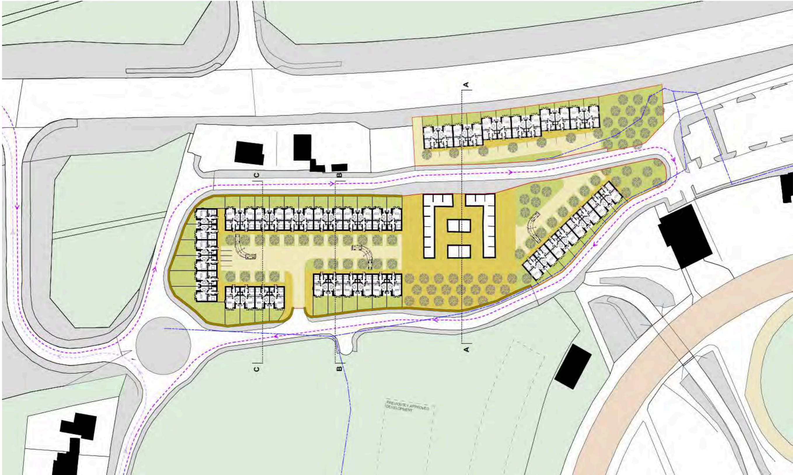
Site Plan of Proposed Retirement Village in the immediate context of Dundalk Stadium as well as showing existing water supply and public sewer network
