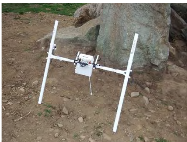
Bartington Grad 601-single axis dual sensor gradiometer.
