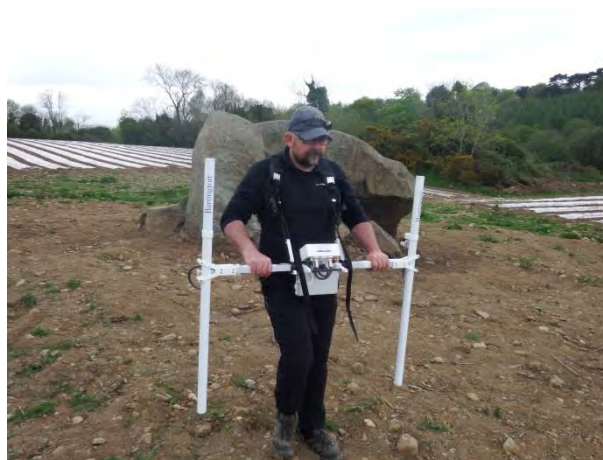
Bartington Grad 601-single axis dual sensor gradiometer.
